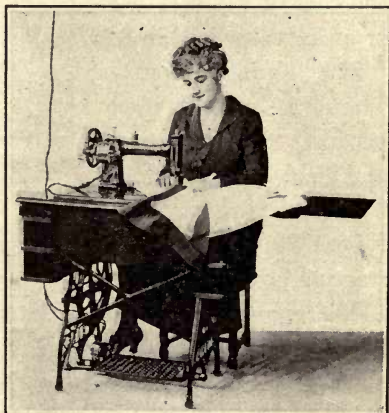
FIGURE 204.—A SMALL ELECTRIC MOTOR USED TO DRIVE A SEWING MACHINE.
